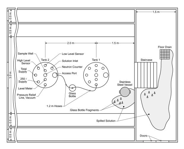
Figure 23. Plan view of the tanks involved in the accident.
