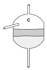
Figure 26. Solution transfer as reconstructed from the transparent plastic mockup of the transfer vessel. Configuration (B) is the postulated state at the time of the accident.
