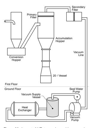
Figure 20. Layout of  $\mathrm{UF}_6$  to uranium oxide conversion equipment and associated vacuum system.
