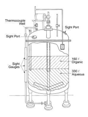
Figure 11. Configuration of solutions (aqueous and organic) in the vessel before the accident.
