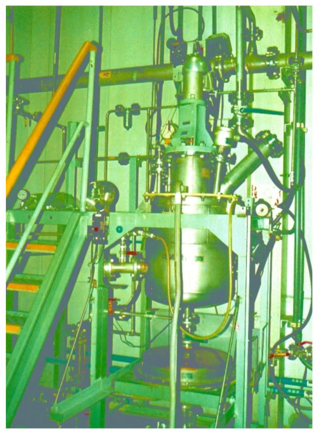
Figure 35. The precipitation vessel in which the process criticality accident occurred.
