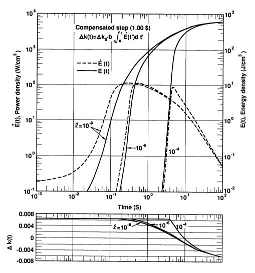
Figure 64. Energy model computation of power vs time. The initial reactivity is 1.0 \$ above delayed critical. Neutron lifetime values are 10-8, 10-6, and 10-4 seconds. The bottom panel shows the corresponding curves of reactivity vs time.
