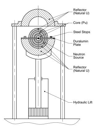
Figure 46. FKBN and assembly involved in the 9 April 1953 accident.
