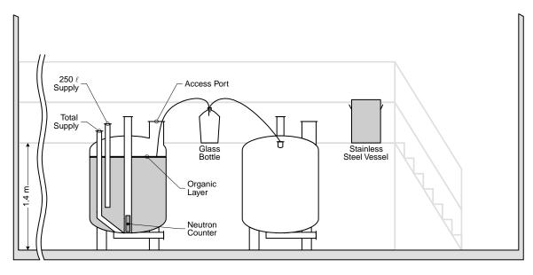
Figure 24. Elevation view of the tanks involved in the accident.
