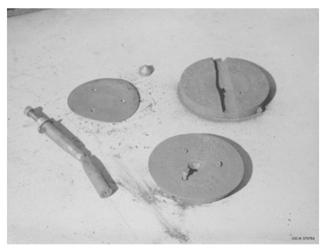
Figure 50. Burst rod and several sections of Lady Godiva showing oxidation and warpage that accompanied the second accident, 12 February 1957.
