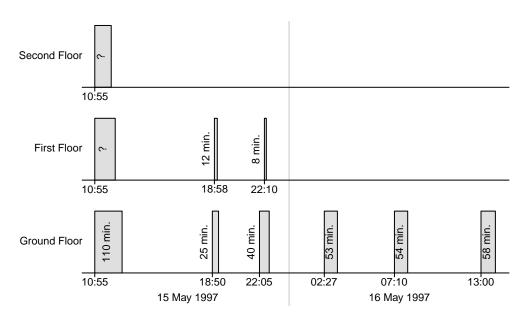
Figure 33. Sequence of alarms and duration that the radiation levels exceeded the alarm level (36 mR/h).
