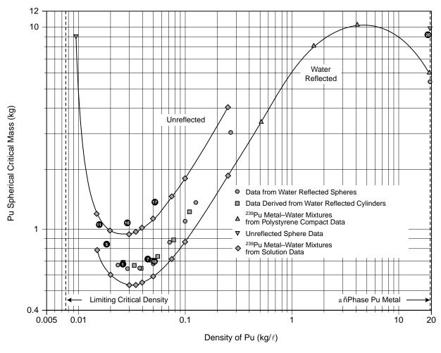
Figure 39. Critical masses of homogeneous water moderated plutonium spheres. The points suggesting an intermediate curve apply to water reflected  $Pu(No_3)_4$  solution with 1 N HNO $_3$  and 3.1%  $^{240}Pu$  content. The accidents are shown by numbered circles.
