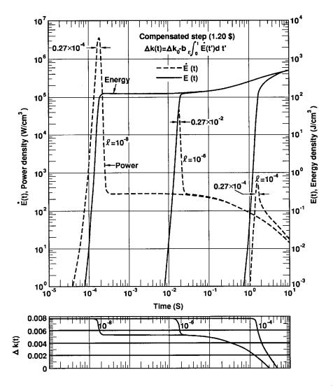
Figure 63. Energy model computation of power and energy release vs time. The initial reactivity is 1.2 \$ above delayed critical. Neutron lifetime values are  $10^{-6}$ ,  $10^{-6}$ , and  $10^{-4}$  seconds. The bottom panel shows the corresponding curves of reactivity vs time.
