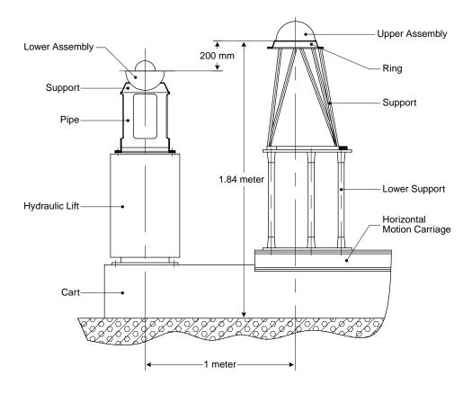
Figure 55. FKBN-2M experimental layout.
