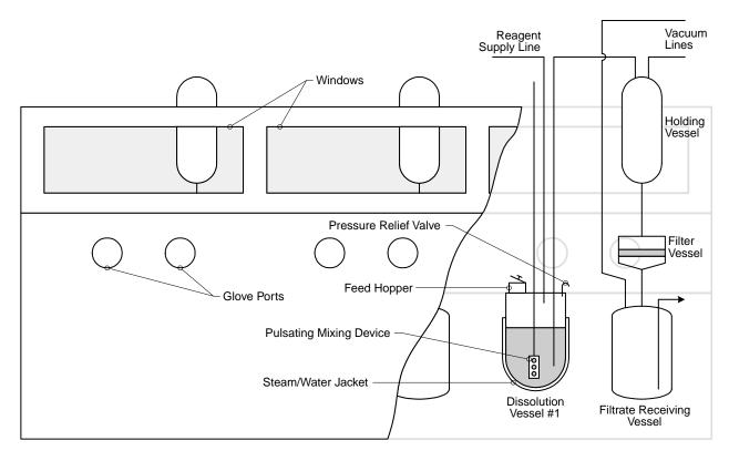
Figure 22. Layout of dissolution glovebox.
