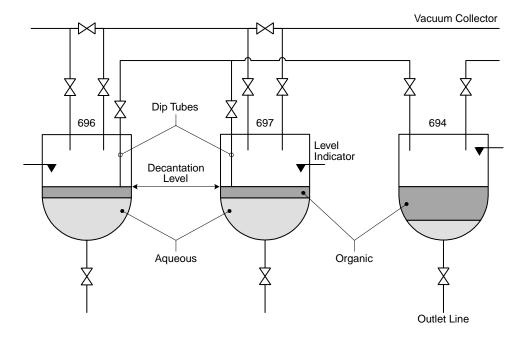
Figure 19. Schematic of vessels showing organic and aqueous solutions (not intended to imply the exact conditions at the time of the accident).
