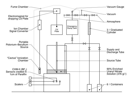
Figure 8. Layout of the experimental equipment.
