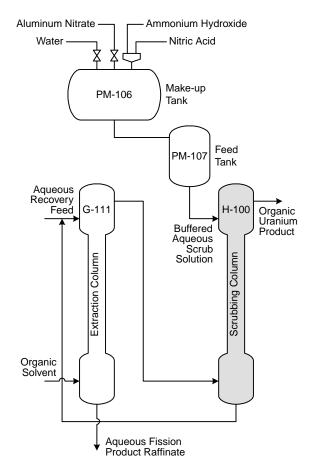
Figure 27. First cycle extraction line equipment. The accident occurred in the lower disengagement section of the H-100 column.
