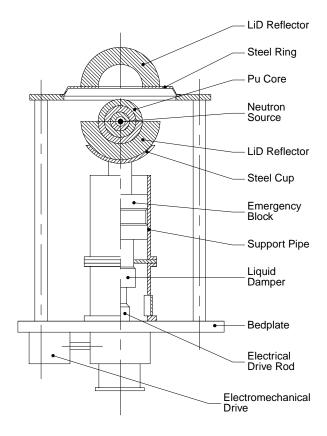
Figure 51. MSKS and assembly involved in the 11 March 1963 accident.
