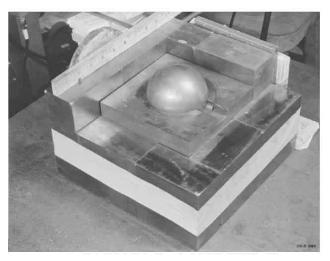
Figure 41. Plutonium sphere partially reflected by tungsten-carbide blocks.
