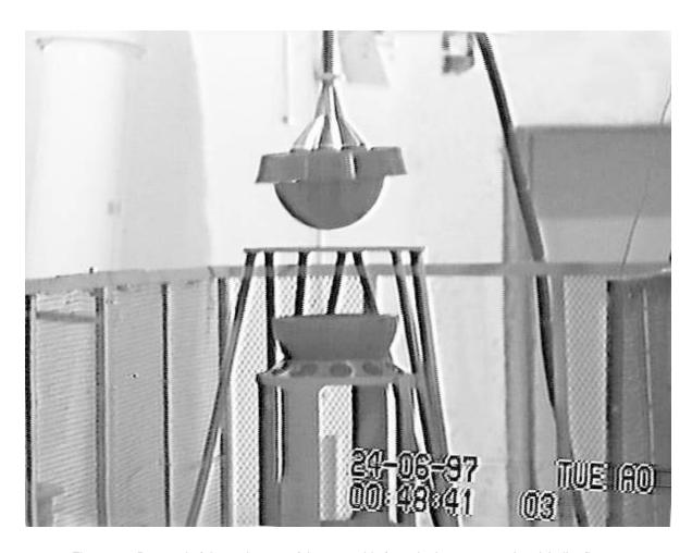
Figure 58. Removal of the main core of the assembly from the lower copper hemishell reflector.
