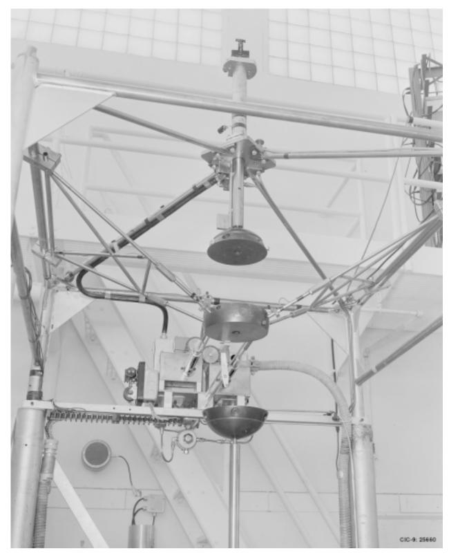
Figure 48. The Los Alamos Scientific Laboratory Lady Godiva assembly (unreflected enriched-uranium sphere) in the scrammed configuration.
