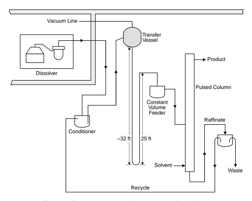
Figure 25. Process equipment related to the criticality accident.
