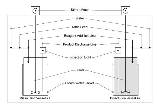
Figure 17. Layout of glovebox equipment.
