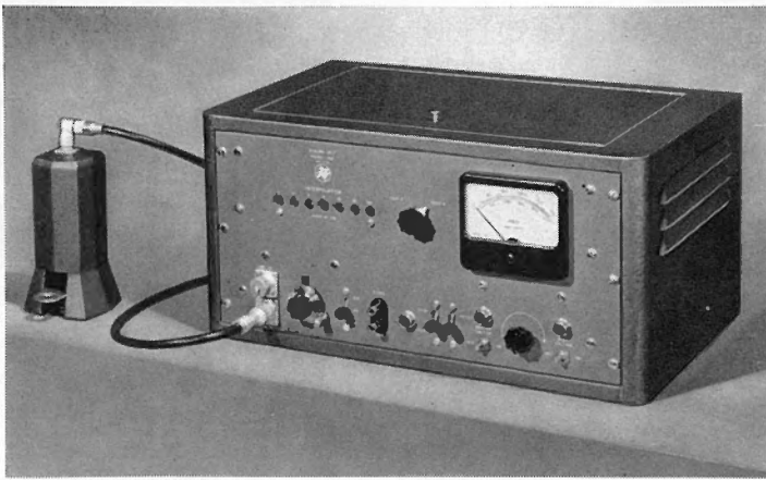
Model 162 Scaler with Model M2 Mount and Model D31 Geiger Counter.
