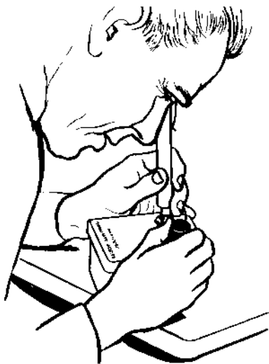
FIGURE 1. — METER HELD IN ZEROING (CHARGING) POSITION ON CHARGER CD V-756
