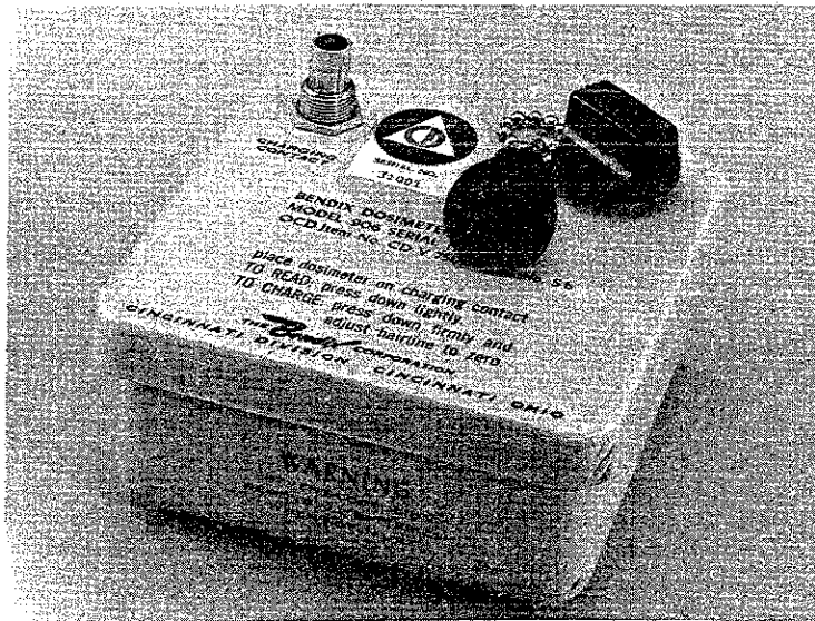
Figure 3-8. A charger with the knob removed from the charging contact.
