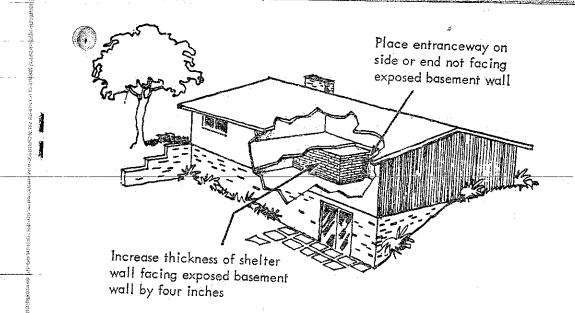
If your basement ceiling is near ground level on three sides and exposed on one side (as with "walk-in" basements), the concrete block shelter (Plan C) must be modified to achieve the desired effectiveness. The following changes should be made:
