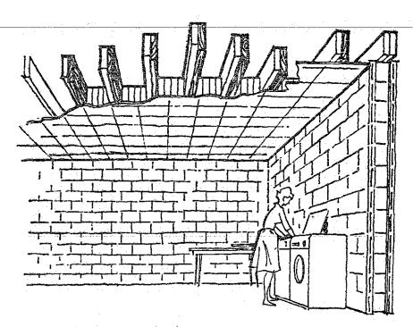
If you need a minimum shelter which will not interfere with an existing corner of your basement, try this plan. It is so arranged that the shelter area can be enlarged at either end, depending upon the size of the basement.
