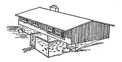
Enclosing your patio area with a solid masonry screen wall will give you privacy for lounging and cook-outs, and will provide a barrier shield to increase the PF in the basement area.
