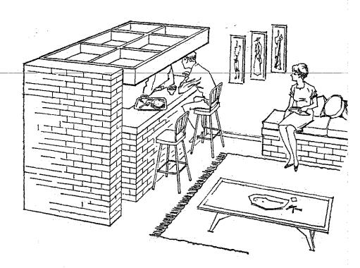
A snack bar built of brick or block can be converted into a fallout shelter in a short period of time by lowering a strong hinged false ceiling to rest on the snack bar.
