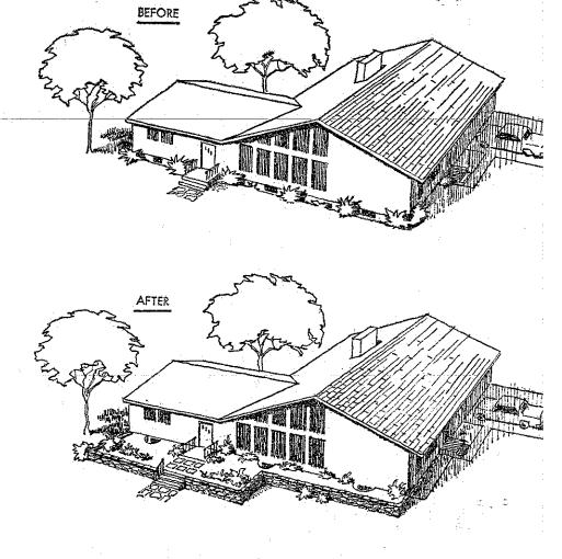
Where basements are not completely belowgrade, here are some additional ideas which can be used to increase the shielding of exposed basement walls. A brick, masonry, or stone planter box along one or more sides of the house will improve protection substantially, and will provide an attractive setting for shrubs and flowers as well. If the partially exposed wall is at the rear or side of the house, an elevated garden could be built with masonry retaining walls.
