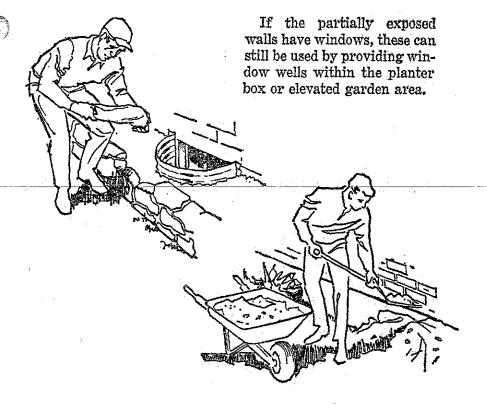
Your basement's PF will also be increased by providing additional shielding to the exposed section. This can be done by piling patio block, sand, earth, cordwood or similar materials against the exposed wall.
