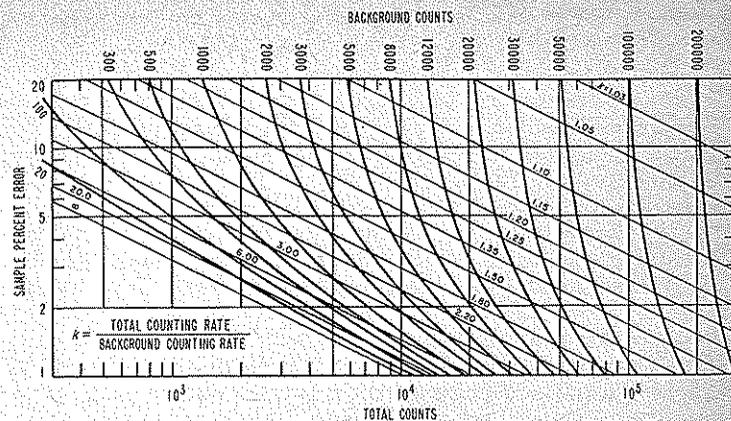
FIGURE 2.5-1. Relationship between precision and number of observed counts taking account of background.
