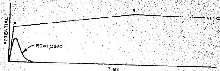
FIGURE 2.1-2. Voltage pulse on collecting electrode of pulse ionization chamber.
