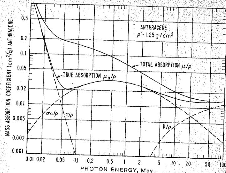
FIGURE 2.4-2. The  $\gamma$ -ray mass-absorption coefficients of anthracene versus  $\gamma$ -ray energy.
