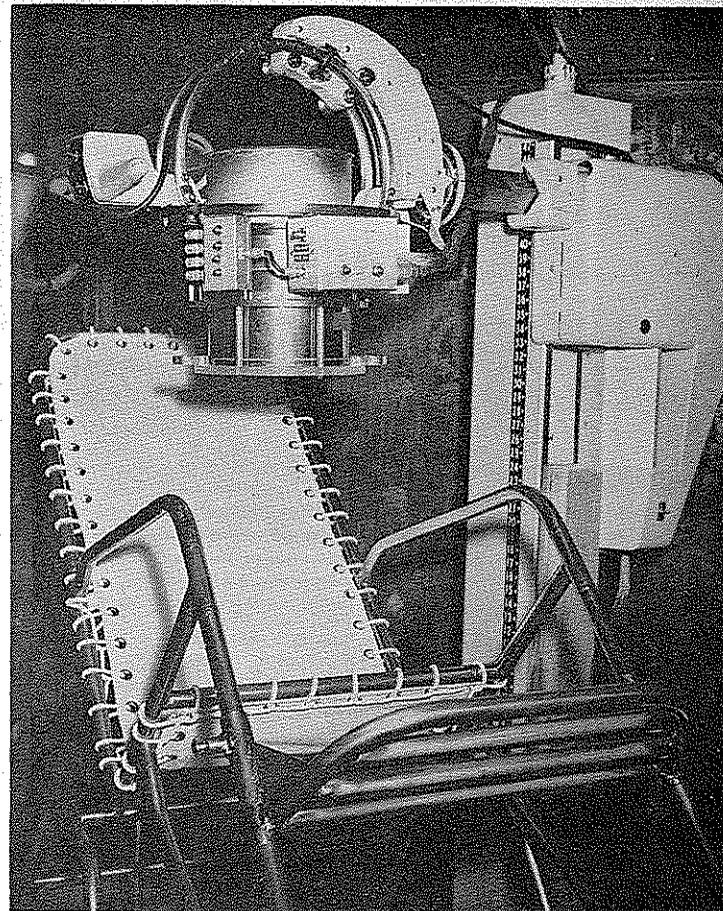
FIGURE 9.4-3. The 8 × 4-inch sodium-iodide crystal in the Walter Reed Army Institute of Research steel room.
