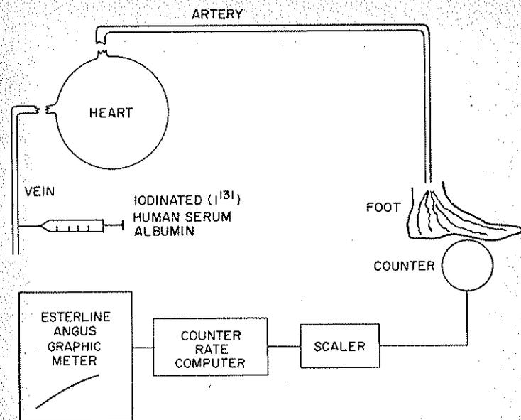
FIGURE 11.2-1. Schematic diagram of experiment to measure peripheral vascular flow.
