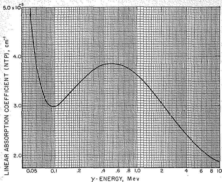
FIGURE 3.6-1. Linear energy absorption coefficient for photons in air at NTP.
