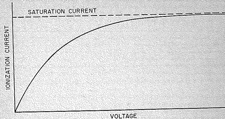
FIGURE 2.1-1. Saturation curve (ion current versus collecting voltage) for a typical ionization chamber.
