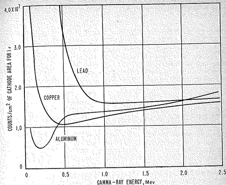
FIGURE 3.6-4. Response of Geiger-Müller counters of different cathode materials in terms of gamma dose in roentgens. [Hine and Brownell, 1956, ch. 5, Geiger-Müller counters and proportional counters, W. K. Sinclair; courtesy of Academic Press.]
