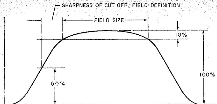
FIGURE 9.2-1. Transmission of collimator as determined by moving a point source of radiation on a plane at the working distance.
