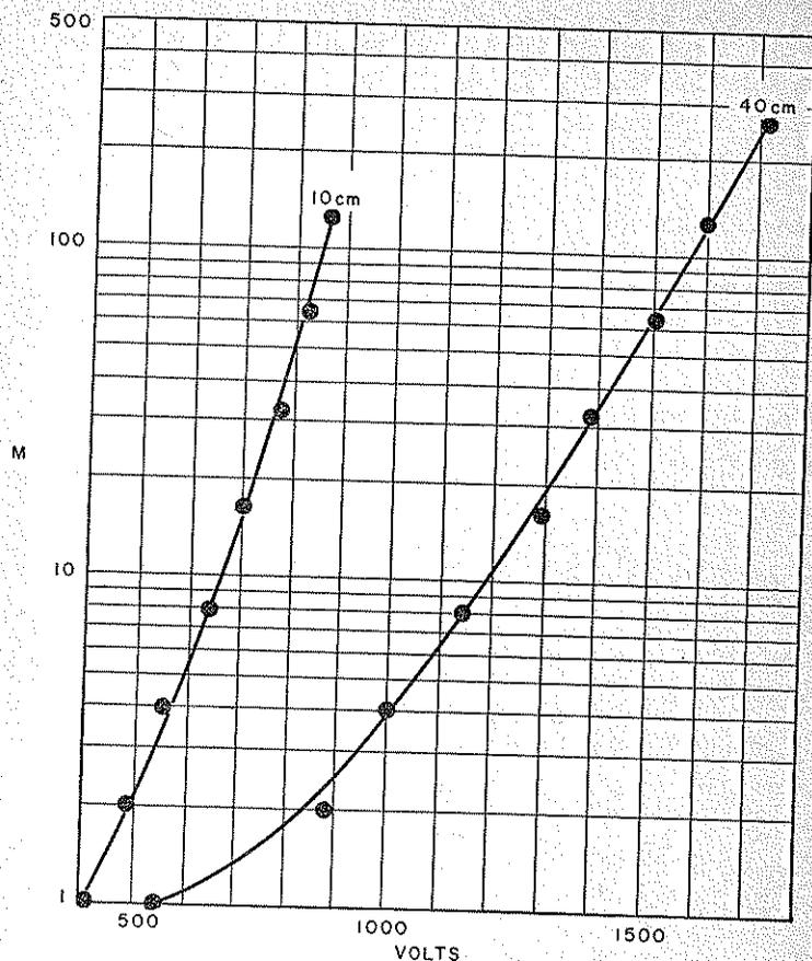
FIGURE 2.2-1. Multiplication factor,  $M$ , as function of applied voltage for argon at pressures of 10 and 40 cm Hg, radius of center wire = 0.005 in., radius of outer electrode = 0.435 in. [Segré, 1953, pt. I, Detection methods, H. H. Staub; courtesy of John Wiley & Sons, New York, N.Y.]
