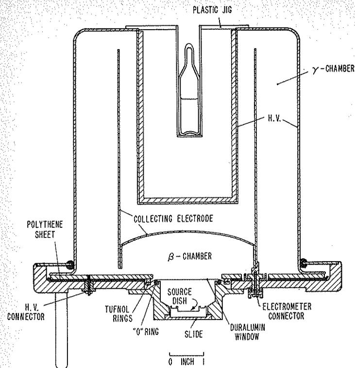
FIGURE 7.2-2. Combined beta-gamma reference ionization chamber.
