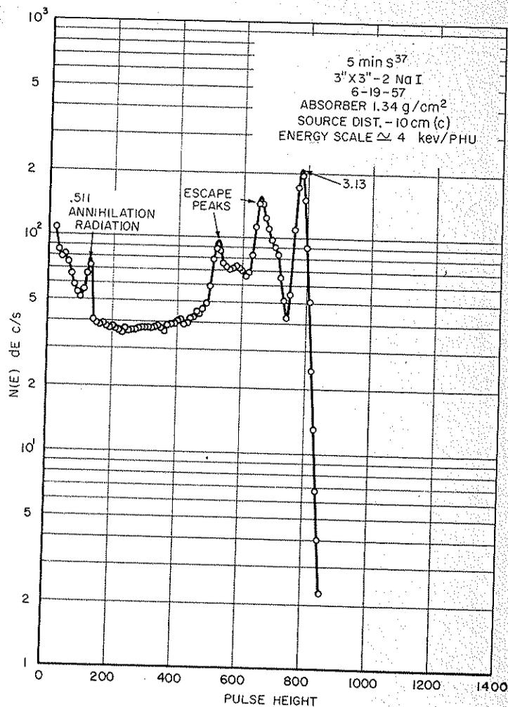
FIGURE 2.4-6. Pulse-height distributions for 3.13-Mev gamma rays incident on a thallium-activated sodium iodide crystal. [Heath, 1957; courtesy of U.S. Atomic Energy Commission.]
