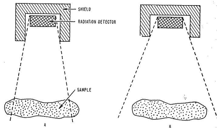
FIGURE 9.1-3. Shielding of an uptake counter.
