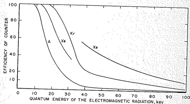
FIGURE 2.2-3. Percentage of quanta absorbed in 50 mg/cm<sup>2</sup> of argon, krypton, and xenon (i.e., 5-cm path at 5 atmospheres in argon, at 2.5 atmospheres in krypton, or at 1.5 atmospheres in xenon). [Curran, 1950; courtesy of Atomic World, formerly Atomics.]
