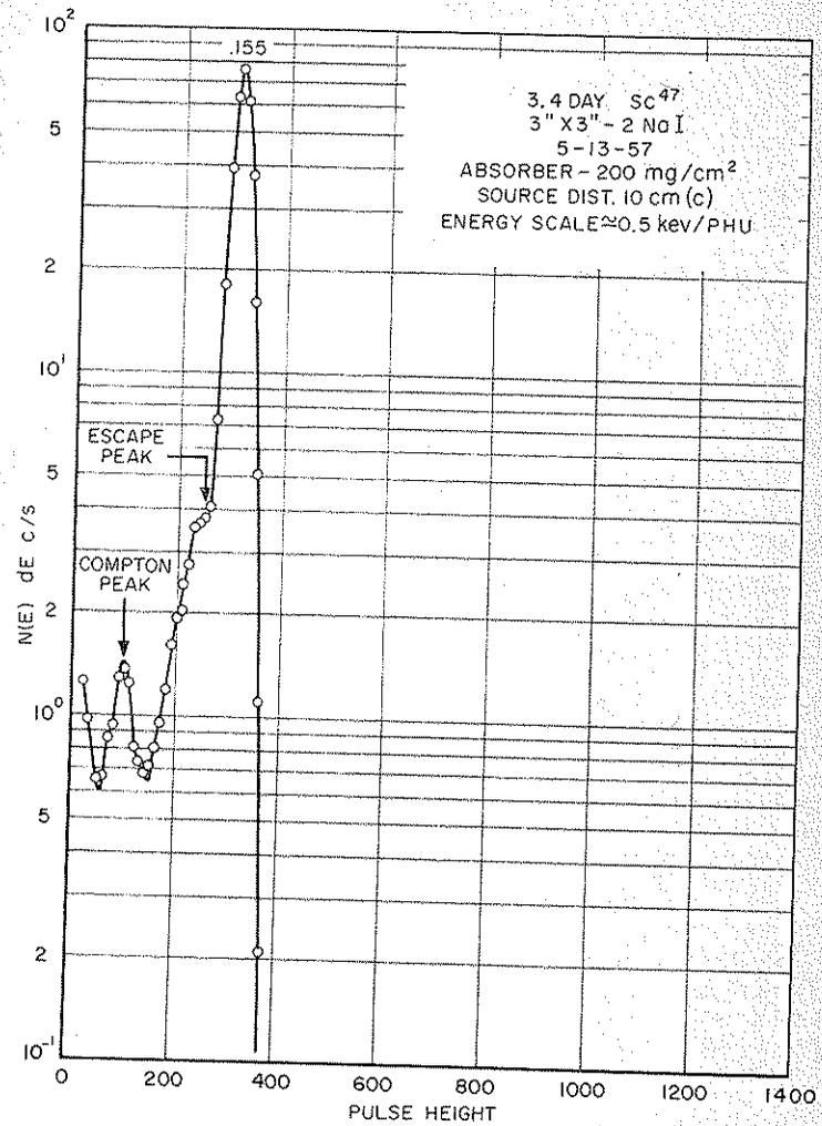
FIGURE 2.4-4. Pulse-height distributions for 0.155-Mev gamma rays incident on a thallium-activated sodium iodide crystal.
