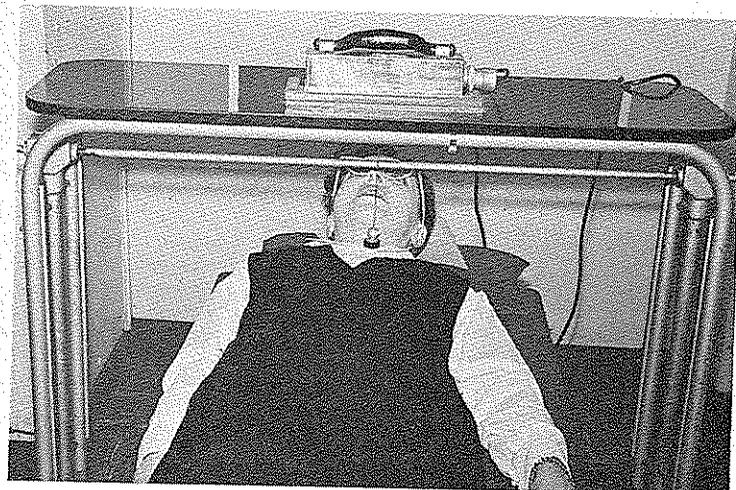
FIGURE 9.1-1. Assembly for uptake measurements using a shielded bismuth-coated Geiger-Müller counter mounted on a hospital over-the-bed table with height adjustable by a crank.
