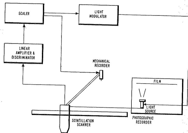
FIGURE 10.3-1. Block diagram of scanner with two types of recording system.
