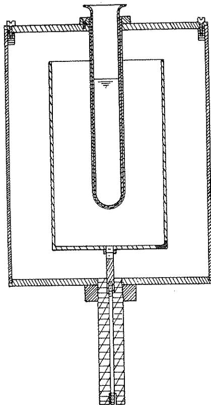
FIGURE 7.2-1. Well-type ionization chamber designed by C. B. Braestrup for the assay of gamma-emitting nuclides.
