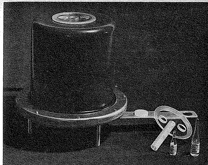
FIGURE 7.2-3. Combined beta-gamma reference ionization chamber with plastic jig for the support of small ampoules.
