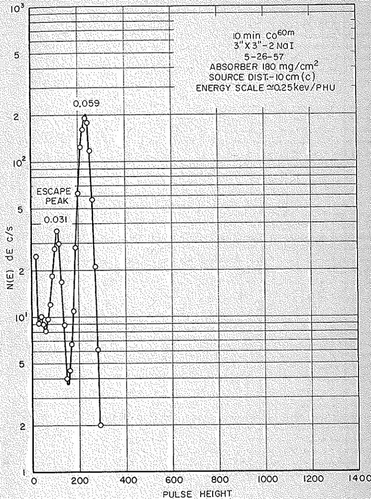
FIGURE 2.4-3. Pulse-height distributions for 0.059-Mev gamma rays incident on a thallium-activated sodium iodide crystal.
