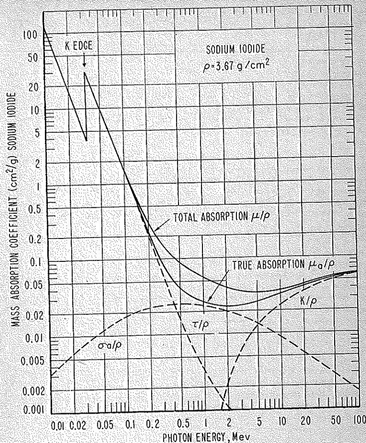
FIGURE 2.4-1. The  $\gamma$ -ray mass-absorption coefficients of sodium iodide versus  $\gamma$ -ray energy. [Hine and Brownell, 1956, ch. 6, Scintillation detectors, W. J. Ramm, courtesy of Academic Press.]
