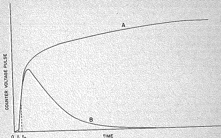
FIGURE 2.2-2. Voltage pulse from proportional counter. [Rossi, 1952; courtesy of Prentice-Hall.]
