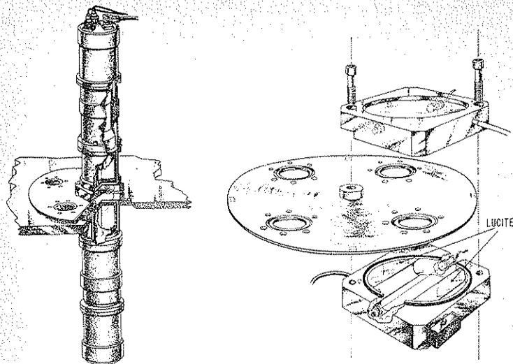
FIGURE 3.2-1. A  $4\pi\beta\text{-}\gamma$  coincidence counting unit. Left, the complete assembly, excluding shielding. Right, an exploded view of the  $4\pi\beta$  proportional gas-flow counter.
