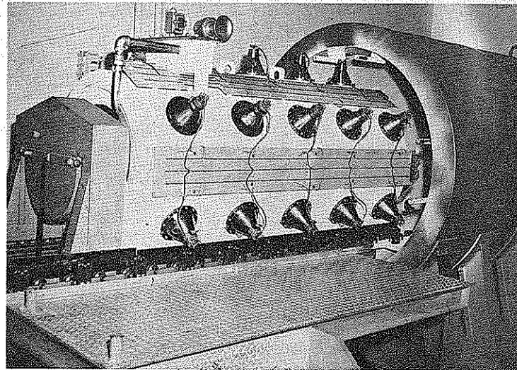
FIGURE 9.4-2. Whole-body liquid scintillation counter at the Walter Reed Army Institute of Research with the detector tank partially withdrawn, showing some of the 30 5-inch photo-electron multiplier tubes.
