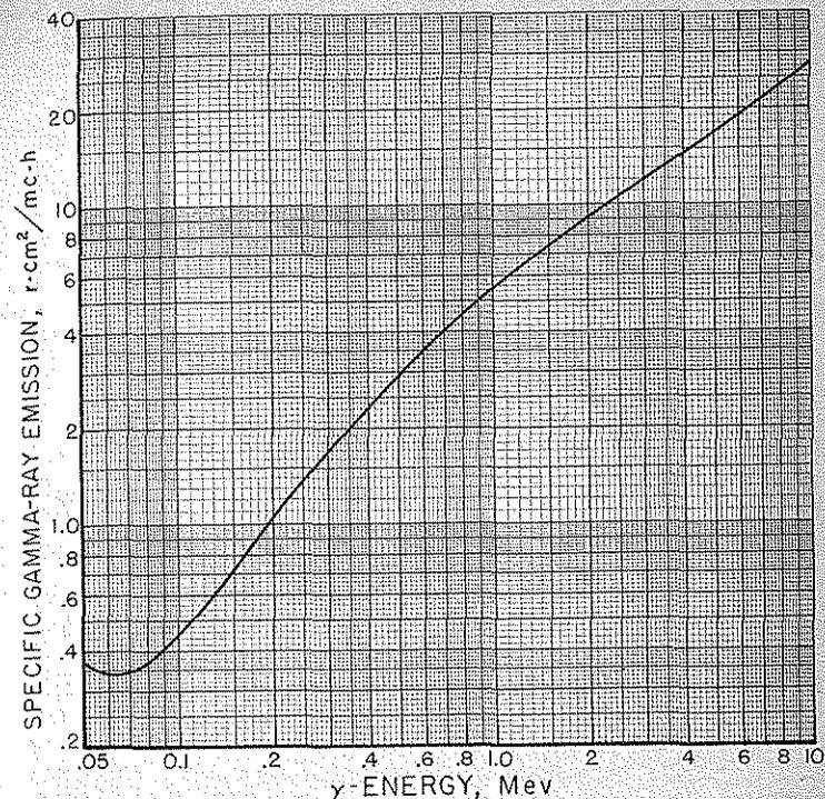
FIGURE 3.6-2. Specific gamma-ray emission  $\Gamma$  for a point source assuming one photon of energy  $E_\gamma$  per disintegration.
