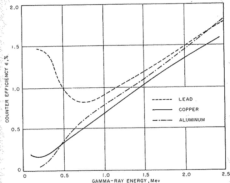
FIGURE 3.6-3. Intrinsic counter efficiency as a function of gamma-ray energy in Geiger-Müller counters with different cathode materials.
