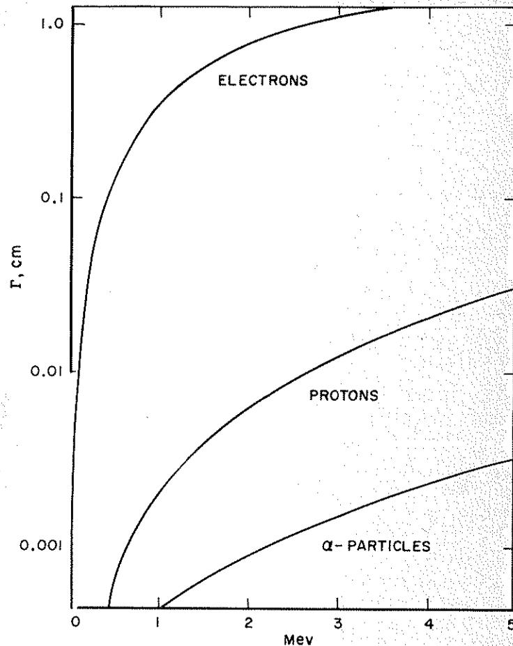
FIGURE 2.4-7. Range-energy curves for ionizing particles in anthracene. [Birks, 1953; courtesy of McGraw-Hill.]
