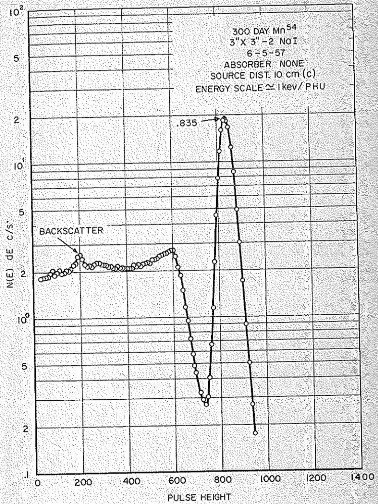
FIGURE 2.4-5. Pulse-height distributions for 0.835-Mev gamma rays incident on a thallium-activated sodium iodide crystal.
