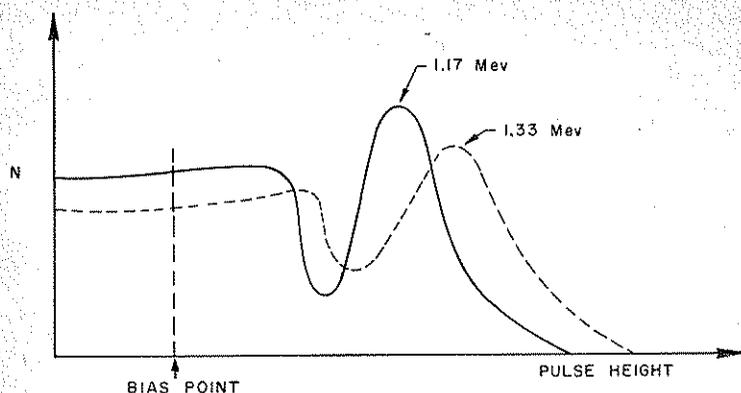
FIGURE 3.2-2. Integral pulse-height curve for gamma rays of 1.17 and 1.33 Mev.
