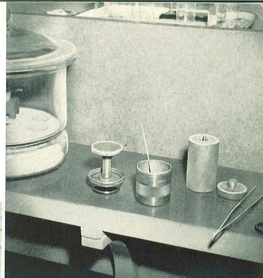
This is the equipment required for handling and crushing the Radium Bromide tubes shown in the first picture.
