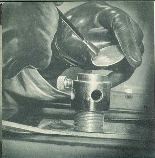
Radium Sulphate is transferred into funnel of filling apparatus which contains the needle in the jig.
