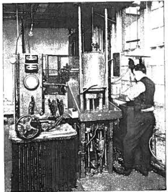
FIG. 3. TREATING BOTTLE AND TRANSFORMER FOR SINTERING TUNGSTEN AND MOLYBDENUM RODS. The operator is lowering the bottle over the rod which is held in place by the heavy copper clamp.
